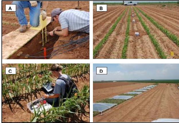
Fig. 1 Installation of TDR sensors for measuring volumetric soil water content in an array above and to each side of the drip lateral (A); field where amendments and sensors are located, corn planted to dry the profile prior to irrigating with SDI (B); measuring soil water content with TDR equipment (C); and treatment sites with "rainout" shelters used while wetting with SDI (D).
